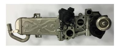
All components are reassembled before the unit is **calibrated** and **tested**. This procedure accurately calibrates the electronic feedback of the valve. The coolant section is then pressure tested to detect any leaks. The final test is to flow gasses through the unit at various pressures and rates to ensure the correct electronic signal is output from the valve
