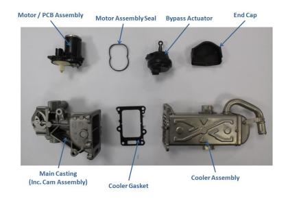
All components are stripped, cleaned of carbon deposits, inspected for wear, and replaced where necessary
